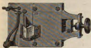
FIG. 50. - Steinheil's slit, showing reflecting prism.
